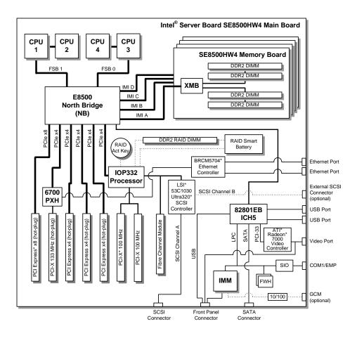
Figure 2. Intel® Server Board Set SE8500HW4 Interconnect Diagram
